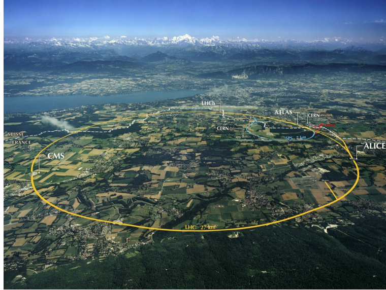
Figure 16: Configuration of the circular accelerator at the Large Hadron Collider (LHC), which spans the border between Switzerland and France. Protons are gradually accelerated over each pass around the 27-km accelerator. Beams of protons are accelerated in each direction: the two beams are then collided at one of four main interaction points. Situated at each interaction point is a detector that studies the debris coming out of the collision. Source: CERN.
